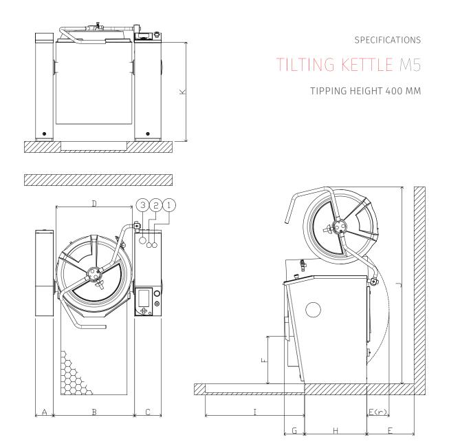
1. COLD WATER, THREAD R15 EXT. PRESSURE (MIN/MAX) 3bar/6bar HARDNESS (MIN/MAX) 3dH/10dH REC. FLOW 25L/MIN 2. HOT WATER, THREAD R15 EXT. PRESSURE (MIN/MAX) 3bar/6bar HARDNESS (MIN/MAX) 3dH/10dH REC. FLOW 11L/MIN TEMPERATURE (MAX) 65° C
